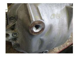
4) Grind away front half of protrusion on top of case.
