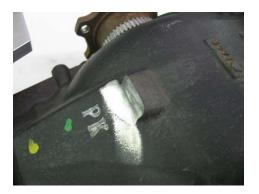
5) R200 Only: Remove rubber/metal isolators from front mounting ears. DO NOT remove R200B isolators.
